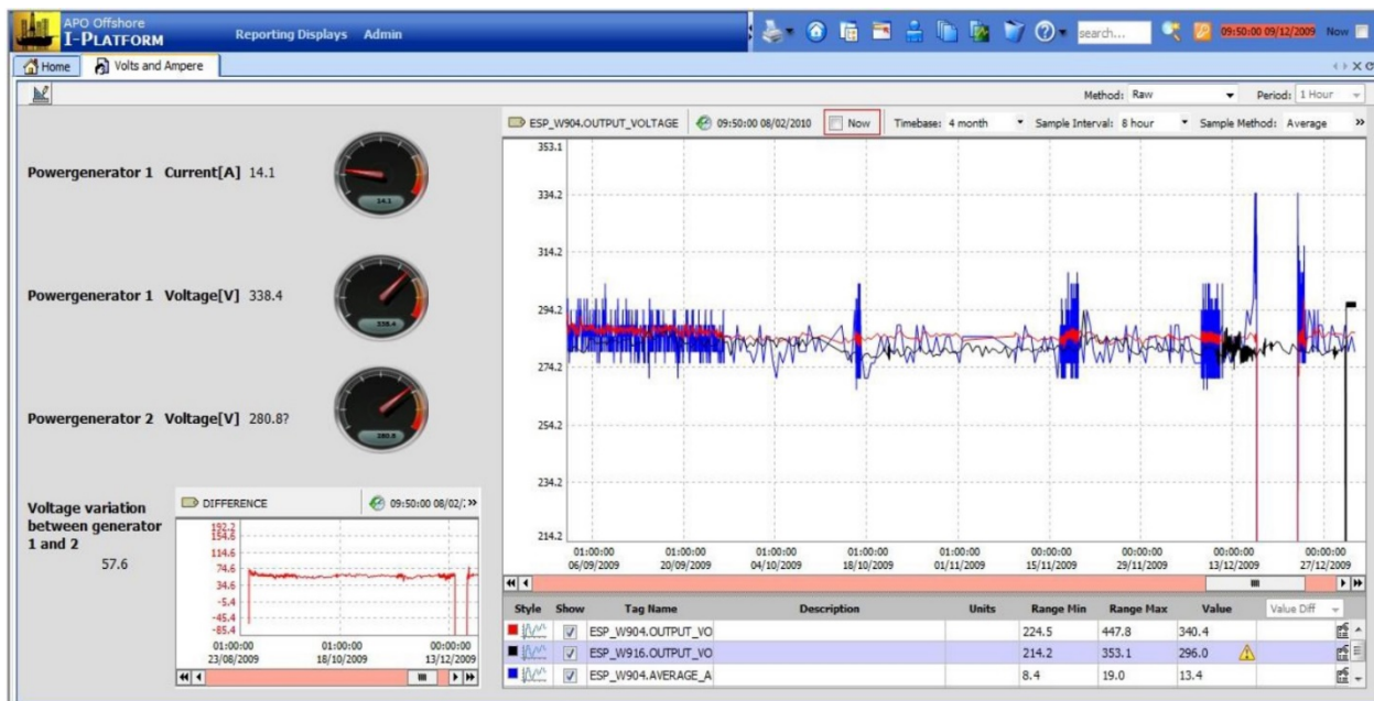
Fig.3. Online display of precursor events to an electric submersible pump failure. While these events would not have triggered static threshold alarms set by the equipment manufacturers, predictive analytics and the output of an artificial neural network were able to use this intelligence to successfully predict the failure. (Data courtesy of APO Offshore, used by permission).
