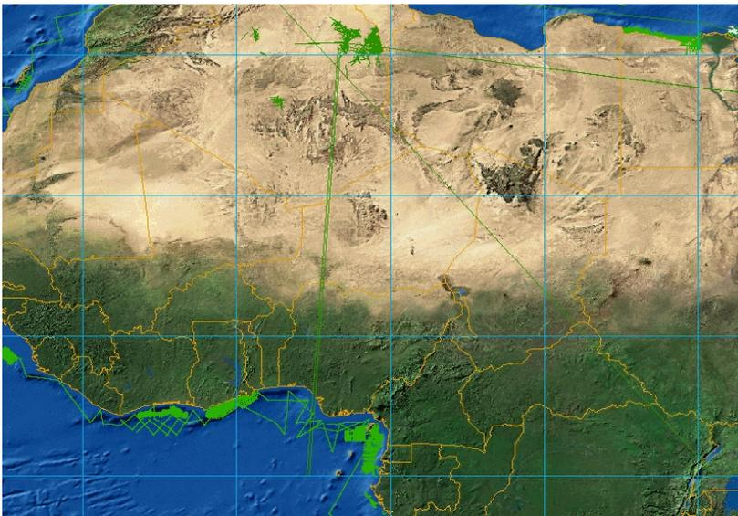
Figure 3: SEG Y data with zero,zero X AND Y's in the trace headers
